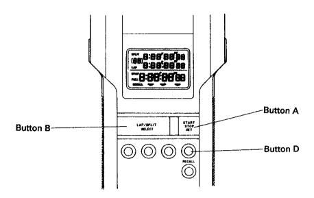
If the stopwatch is left untouched with all the segments lighting up, the display will automatically return to the time/calendar in 1 to 2 minutes. To return to the time/calendar display manually, press button "D".
