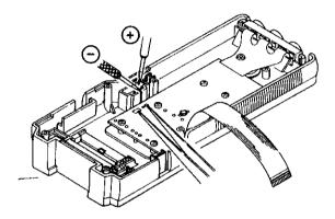
Note: Start measurement 10 seconds after resetting the circuit using the tweezers as illustrated.
